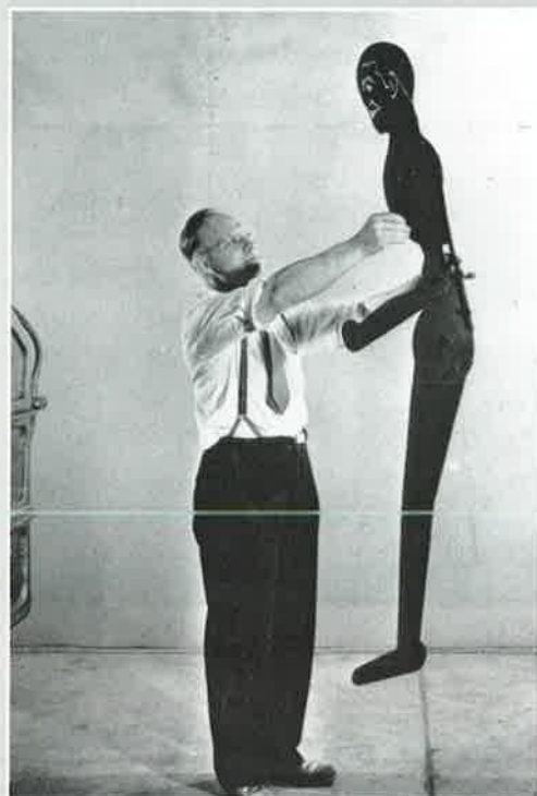
The Thin Man, used to simulate the motions of the human body during crashes.
