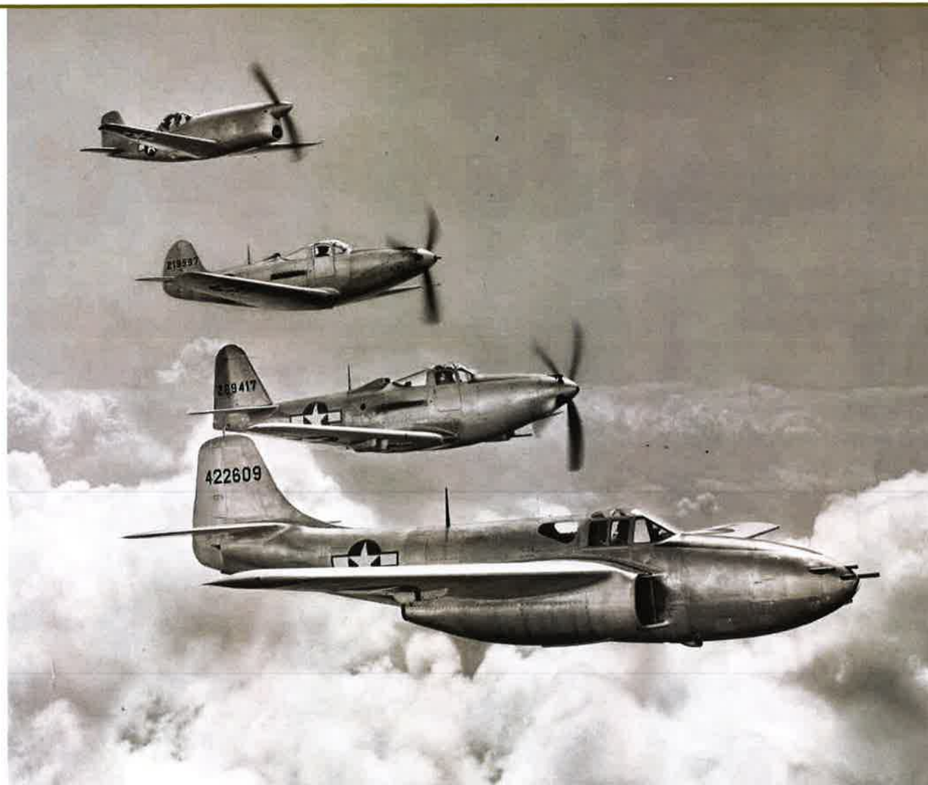
From top to bottom: An XP-77, an experimental fighter made of wood; a P-39; a P-63; and a P-59A – America's first jet fighter.
